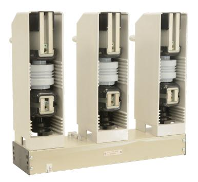
The ISM25\_Shell\_2 Series Circuit Breaker Module has superior characteristics for fast trip applications as well as high-duty switching. The interrupters are driven by three (3) separate magnetic actuators (one per pole) and the module is capable of 30,000 close-open operations at full load.
