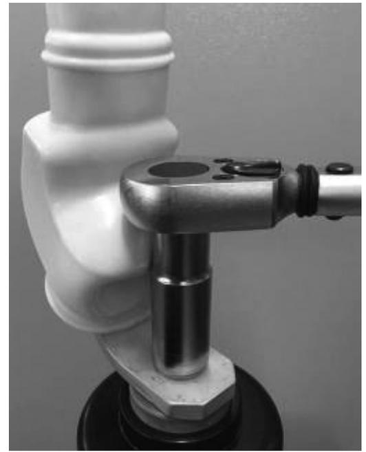
c) screw the bolt M12 with torque
