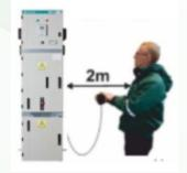
**Remote and safe manual closing** of VCB with a palm-held manual generator. An operator can step aside from the panel front to a safe distance before VCB closing. This totally eliminates the risk of personal injury resulting from a possible internal arc flash.
