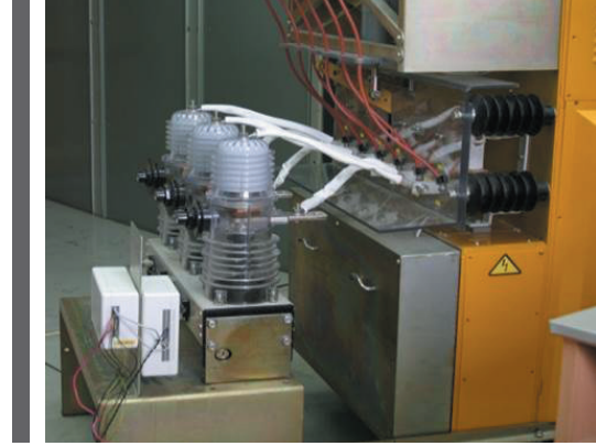
▲ Unit for life testing with rated current of up to 1,600 A
