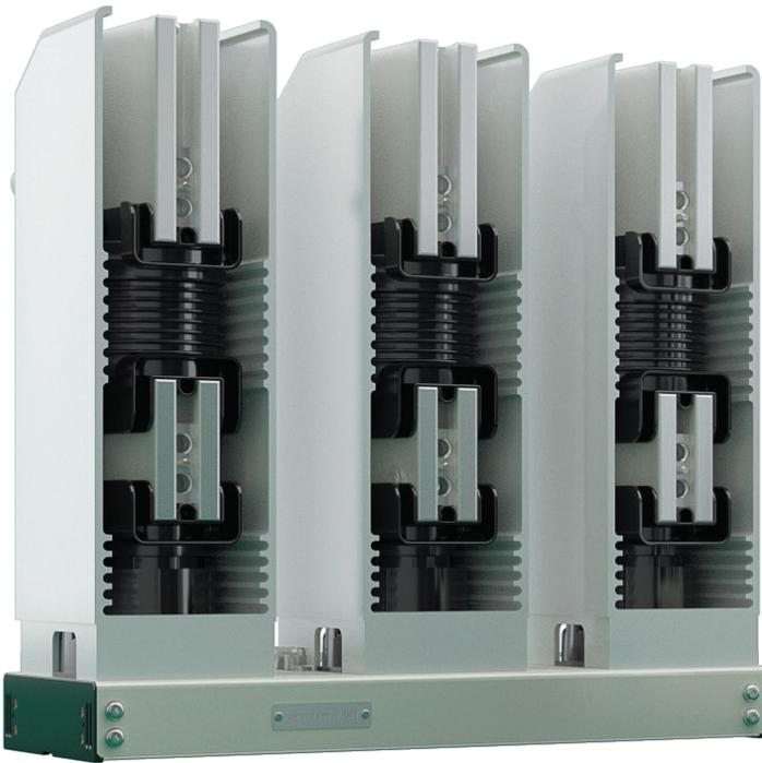
The ISM\_Shell\_2 Series Circuit Breaker Module has superior characteristics for fast trip applications as well as high-duty switching. The interrupters are driven by three (3) separate magnetic actuators (one per pole) and the module is capable of 30,000 close-open operations at full load.
