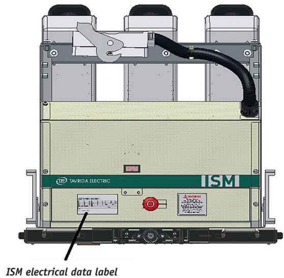
d) VCB25_Shell2_16D labeling
