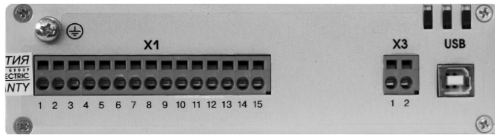
Figure 46 Terminal arrangement of the CM
