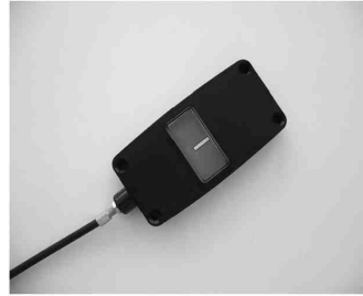
Figure 70 Position indicator shows that main contacts are closed
