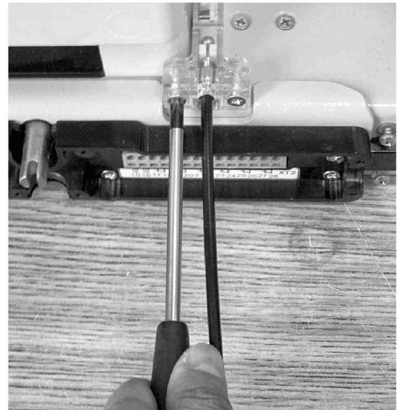
Figure 67 Return the cover and fasten it to the ISM.
