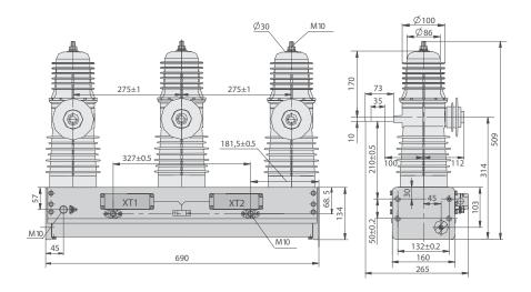
27 kV VCB, PCD 275 mm Weight: 38 kg ISM25\_LD\_1(275)
