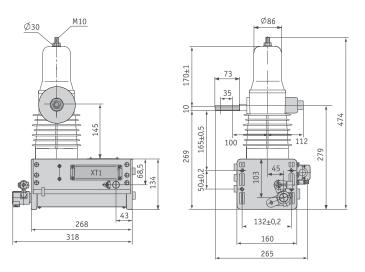
15 kV single-phase VCB, ISM15\_LD\_3 Weight: 13 kg
