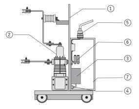
Figure 50 Draw out type installation
