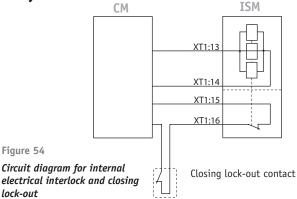
Variant 2 - In the ISM auxiliary switch circuit
