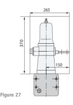
Recommended size and position of the segregation plates for ISM, 15 kV PCD 150 mm
