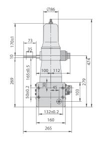
15 kV VCB, PCD 150 mm Weight: 34 kg ISM15\_LD\_1(67)
