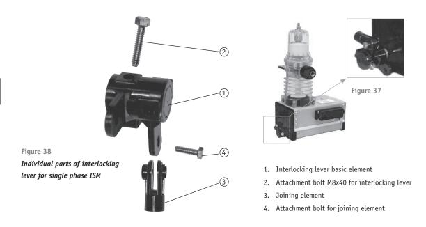
To the joining element (3) a mass M  $\leq$  0.35 kg respectively attached.
