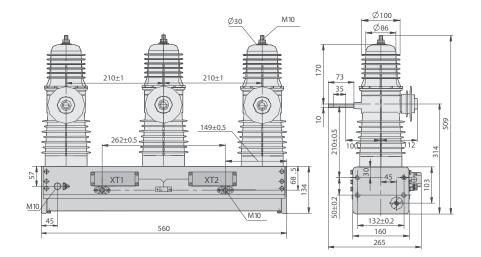
27 kV VCB, PCD 210 mm Weight: 36 kg ISM25\_LD\_1(210)
