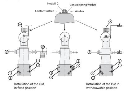
Required fixing points (in each case) Required fixing points (for withdrawable versions) 3 Each two fixing points are required, either 4A+4B or 4A+4C (for fixed installations)
