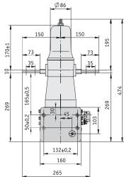
15 kV VCB, continuous busbar, PCD 210 mm Weight: 37 kg By Special Order Only
