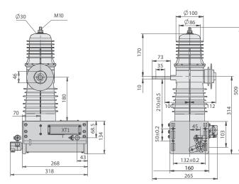
27 kV single-phase VCB, Weight: 13.5 kg
