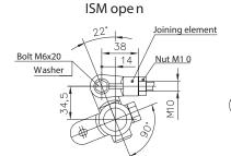
Figure 43 Position of interlocking lever as a function of ISM position
