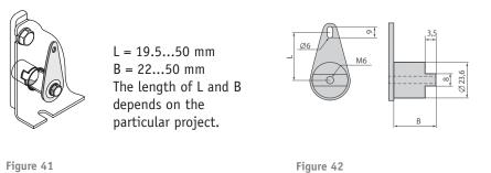
Figure 41 Connection between interlocking lever and synchronizing shaft
