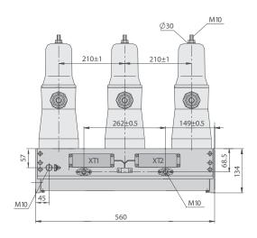
15 kV VCB, PCD 210 mm Weight: 36 kg ISM15\_LD\_1(55)
