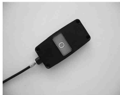
Figure 65 Position indicator shows that main contacts are open
