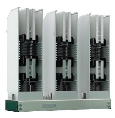
The ISM\_Shell\_2 Series Circuit Breaker Module has superior characteristics for fast trip applications as well as high-duty switching. The interrupters are driven by three (3) separate magnetic actuators (one per pole) and the module is capable of 30,000 close-open operations at full load.
